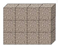
Proppant 1,157 to 1,342 lbs/ft. 12 cubic feet of sand per foot
