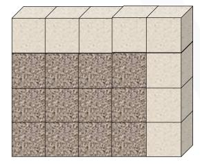
Proppant 1,858 to 1,917 lbs/ft. 20 cubic feet of sand per foot
